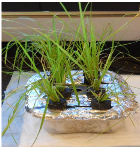
Figure A9: Photograph of reactor used in experiment with soil from Amana colonies and that had cycling of moisture content and redox potential. The switchgrass planted system is used as an example.
